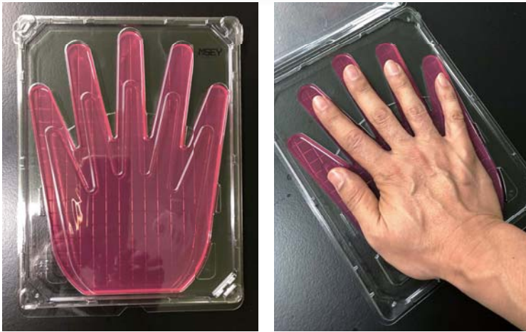
Figure 7: Culture medium for the environmental microorganism test, Hand Petan Check II, mannitol salt agar with egg yolk (EIKEN CHEMICAL Co., Ltd.)
